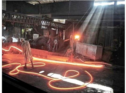
A worker stands around heated steel during the rolling process. **Photo:** The Express Tribune.
