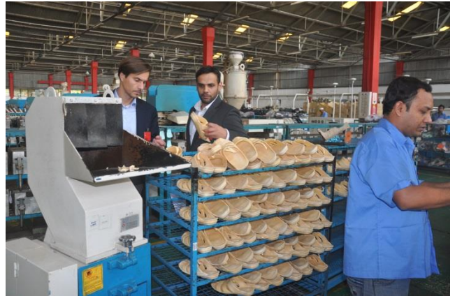
First part of sandal manufacturing, moulded bases being inspected
